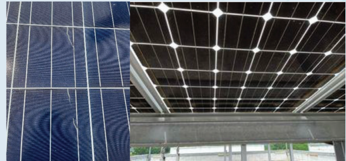
FIGURE 14. DAMAGE TO SOLAR PANELS (LEFT) SOLAR PANELS SEEN FROM BELOW (RIGHT)
